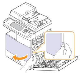
Push the lock lever up and pull the waste toner container out.
